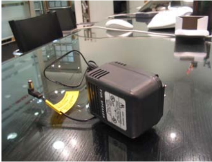
Adaptor(6V 500mA) for Transmitter
