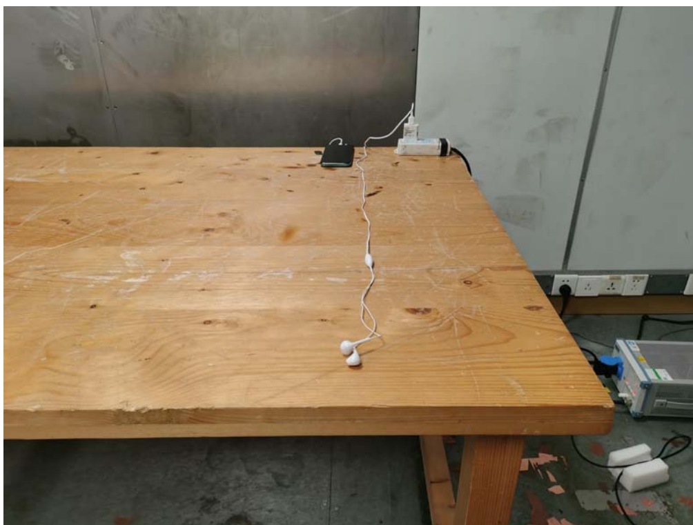
Photo of Radiated Emission Measurement (Below 1G)
