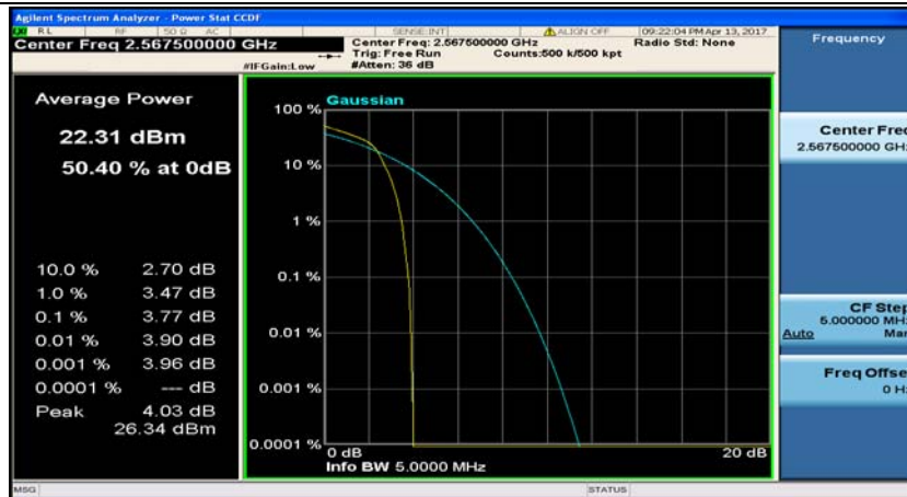
(Channel Bandwidth: 5 MHz)_HCH_16QAM_1RB#24
