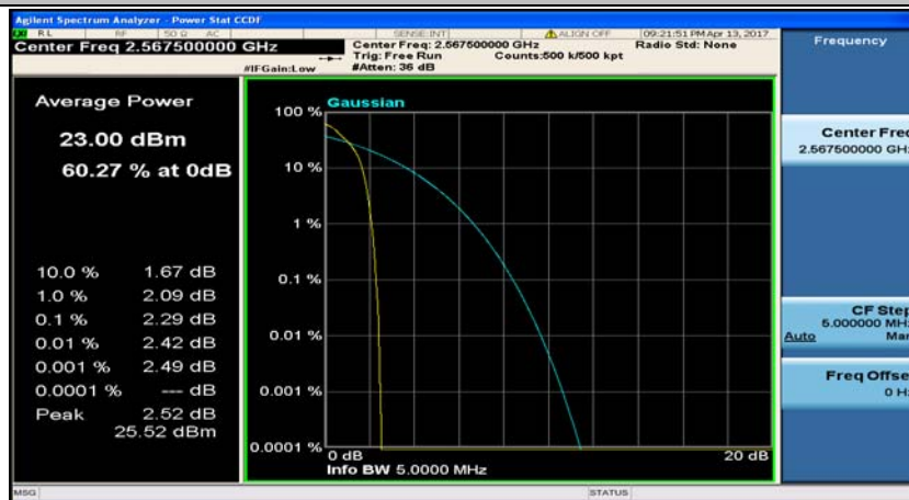
(Channel Bandwidth: 5 MHz)_HCH_QPSK_12RB#0
