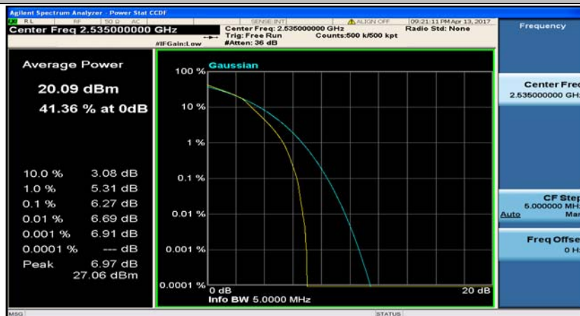
(Channel Bandwidth: 5 MHz)_MCH_16QAM_12RB#13
