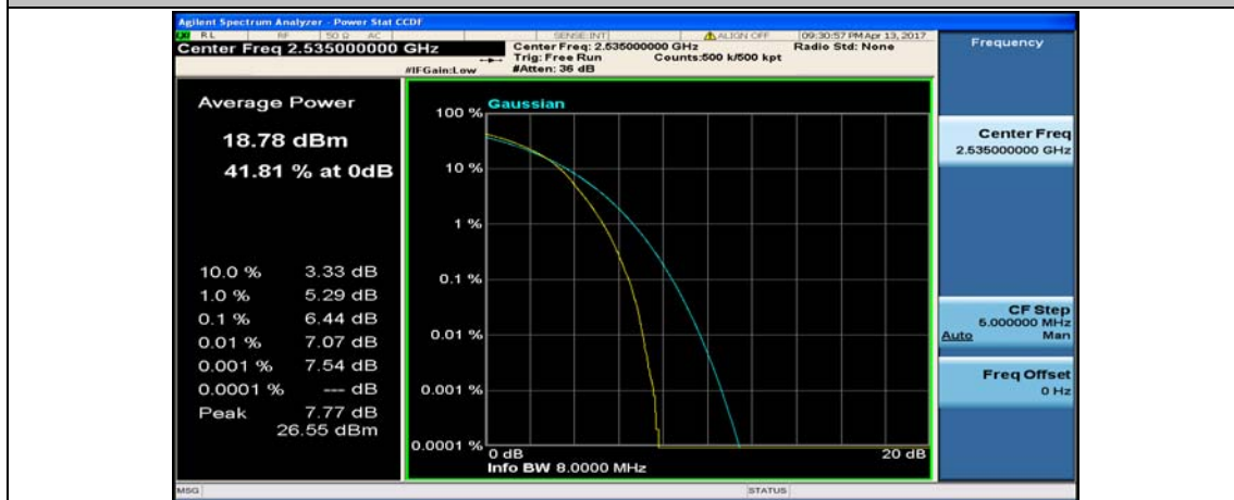
(Channel Bandwidth:15 MHz)_MCH_16QAM_75RB#0
