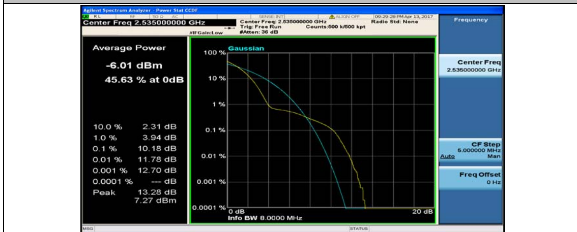
(Channel Bandwidth:15 MHz)_MCH_QPSK_1RB#37
