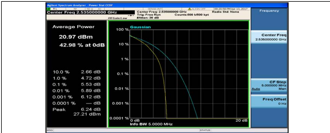
(Channel Bandwidth: 5 MHz)_MCH_QPSK_25RB#0
