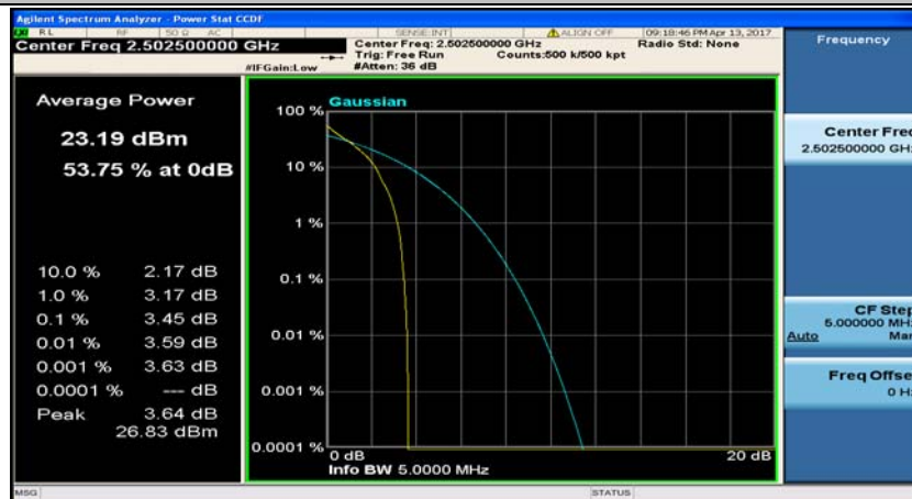
(Channel Bandwidth: 5 MHz)_LCH_QPSK_1RB#24
