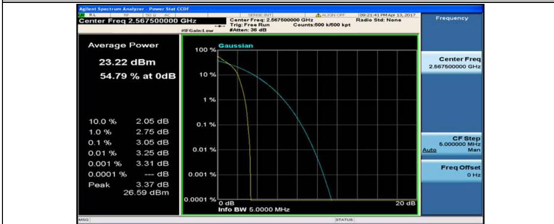
(Channel Bandwidth: 5 MHz)_HCH_QPSK_1RB#12
