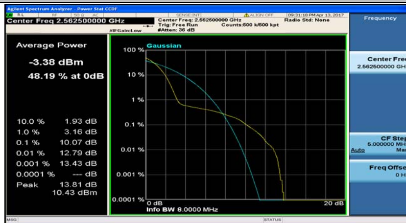
(Channel Bandwidth:15 MHz)_HCH_QPSK_37RB#0
