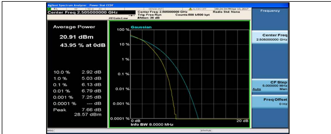
Channel Bandwidth: 10 MHz_MCH_16QAM_1RB#0
