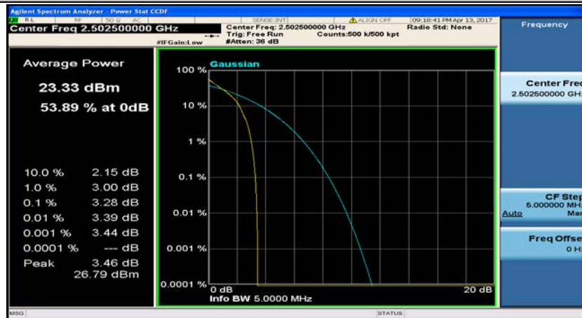
(Channel Bandwidth: 5 MHz)_LCH_QPSK_1RB#12
