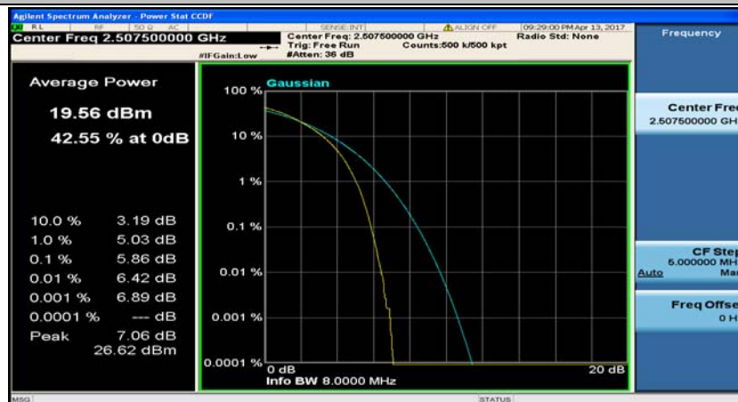
(Channel Bandwidth:15 MHz)_LCH_16QAM_75RB#0
