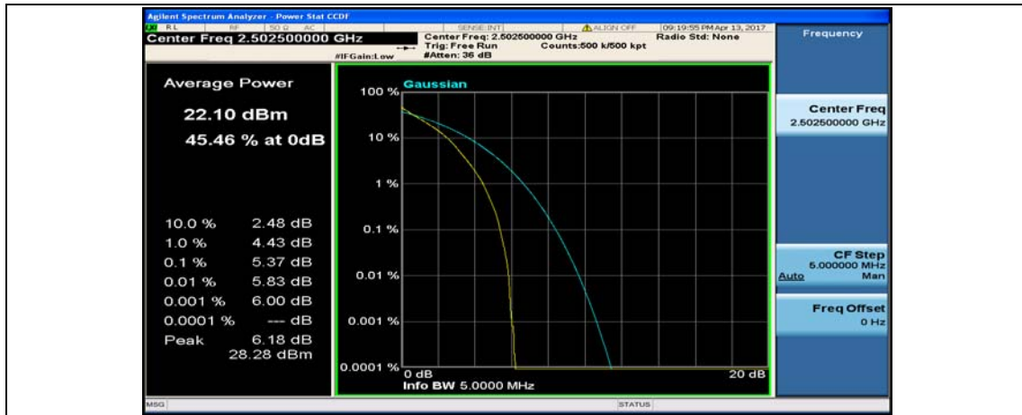
(Channel Bandwidth: 5 MHz)_MCH_QPSK_1RB#0
