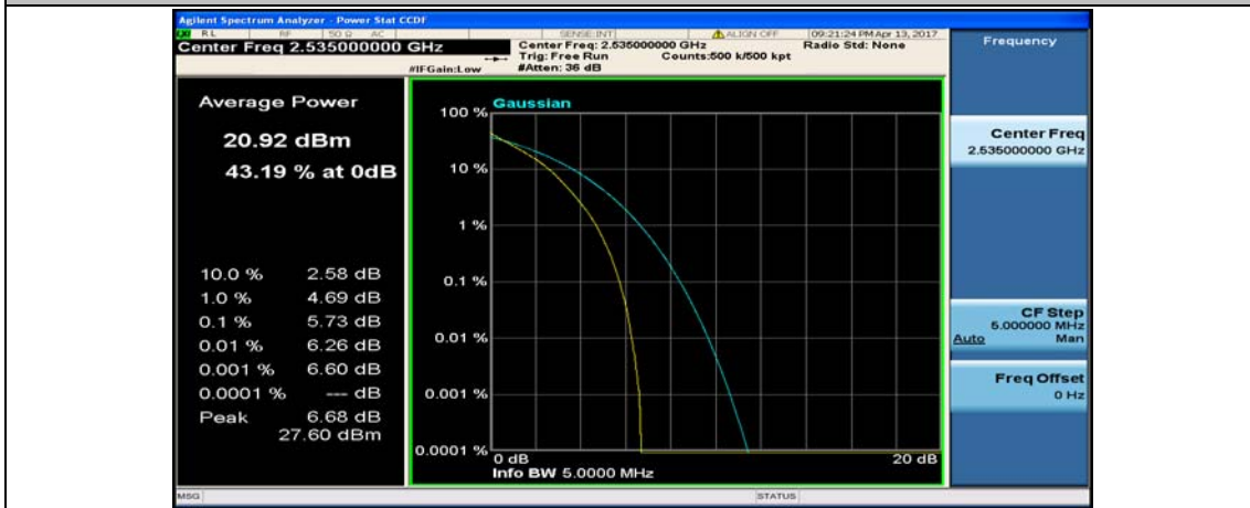
(Channel Bandwidth: 5 MHz)_MCH_QPSK_25RB#0
