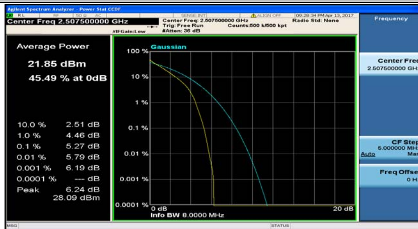
(Channel Bandwidth:15 MHz)_LCH_QPSK_37RB#38
