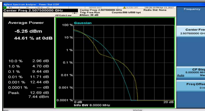
(Channel Bandwidth:15 MHz)_LCH_16QAM_37RB#0
