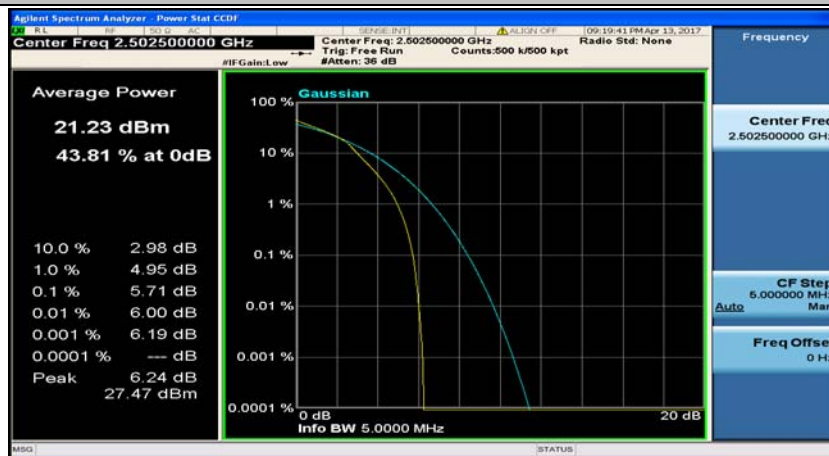
(Channel Bandwidth: 5 MHz)_LCH_16QAM_12RB#13
