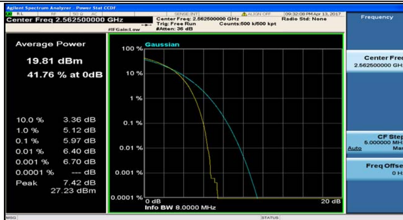
(Channel Bandwidth:15 MHz)_HCH_16QAM_37RB#18
