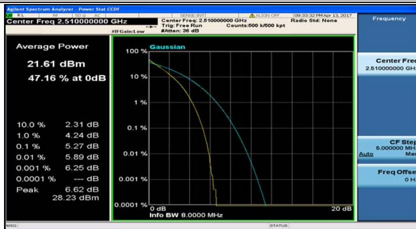
(Channel Bandwidth:20 MHz)_LCH_QPSK_50RB#50
