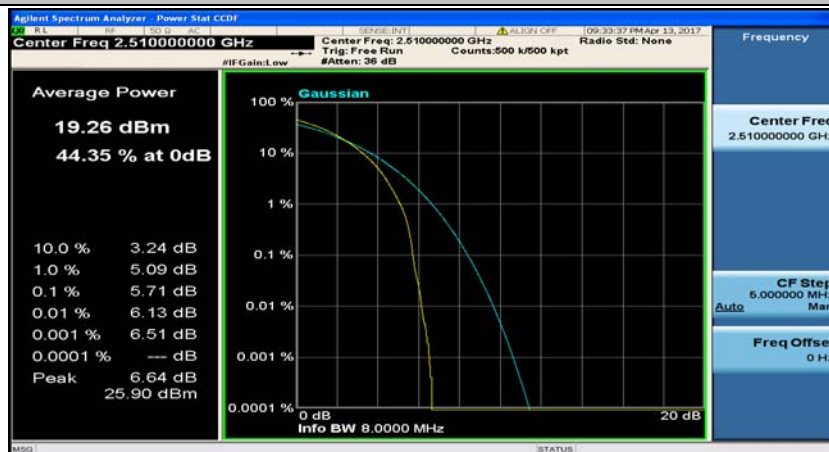
(Channel Bandwidth:20 MHz)_LCH_QPSK_100RB#0
