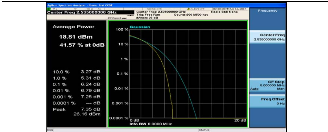
(Channel Bandwidth:15 MHz)_MCH_16QAM_75RB#0
