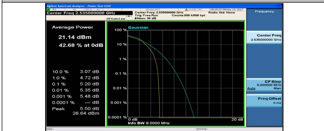
Channel Bandwidth: 10 MHz_MCH_16QAM_1RB#49
