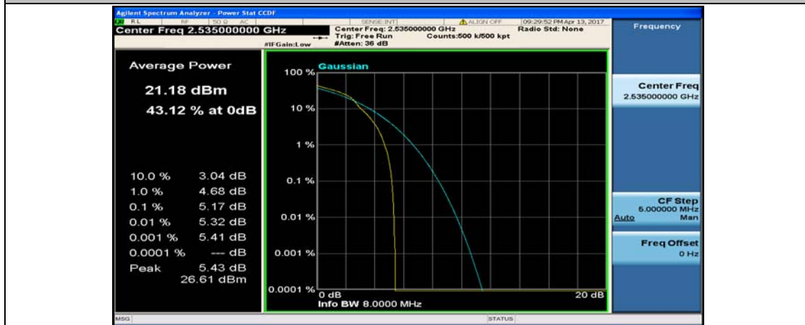
(Channel Bandwidth:15 MHz)_MCH_16QAM_1RB#74
