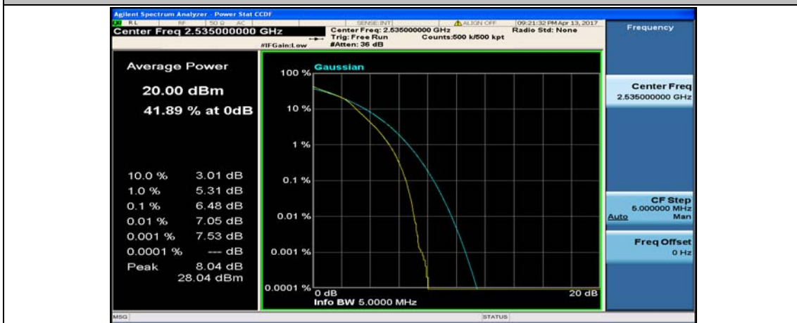
(Channel Bandwidth: 5 MHz)_MCH_16QAM_25RB#0
