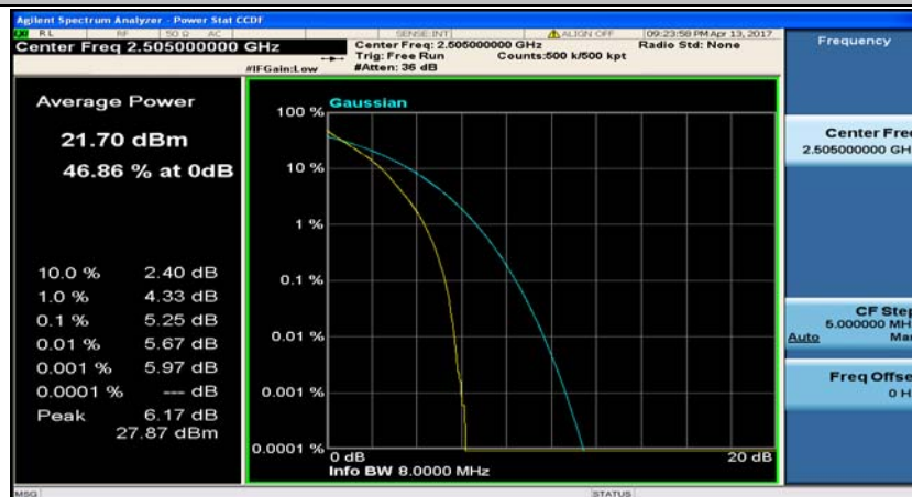
Channel Bandwidth: 10 MHz_LCH_QPSK_50RB#0
