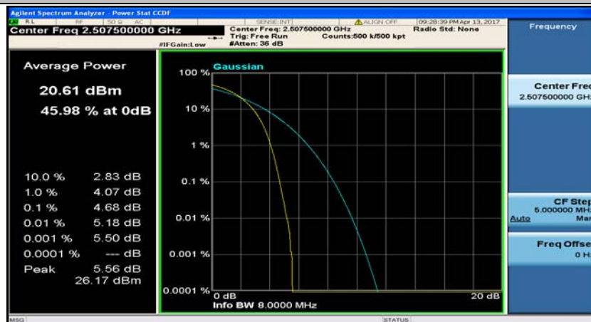
(Channel Bandwidth:15 MHz)_LCH_QPSK_75RB#0
