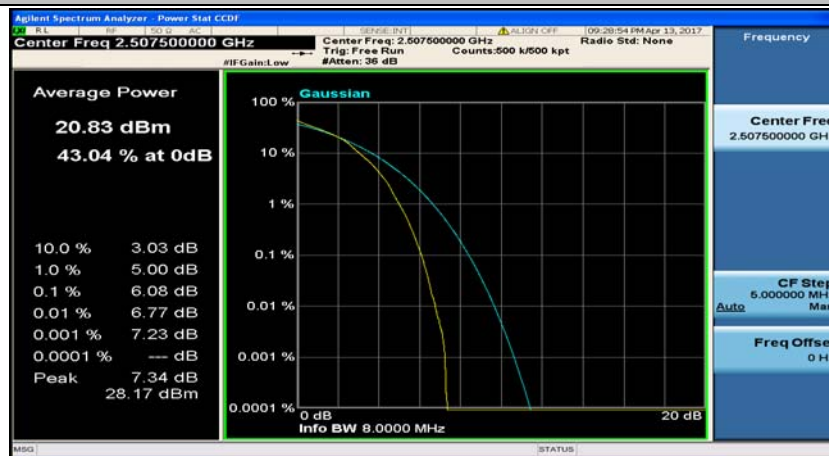
(Channel Bandwidth:15 MHz)_LCH_16QAM_37RB#38
