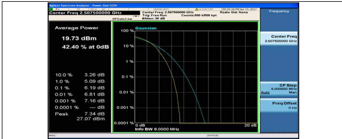
(Channel Bandwidth:15 MHz)_MCH_16QAM_1RB#0
