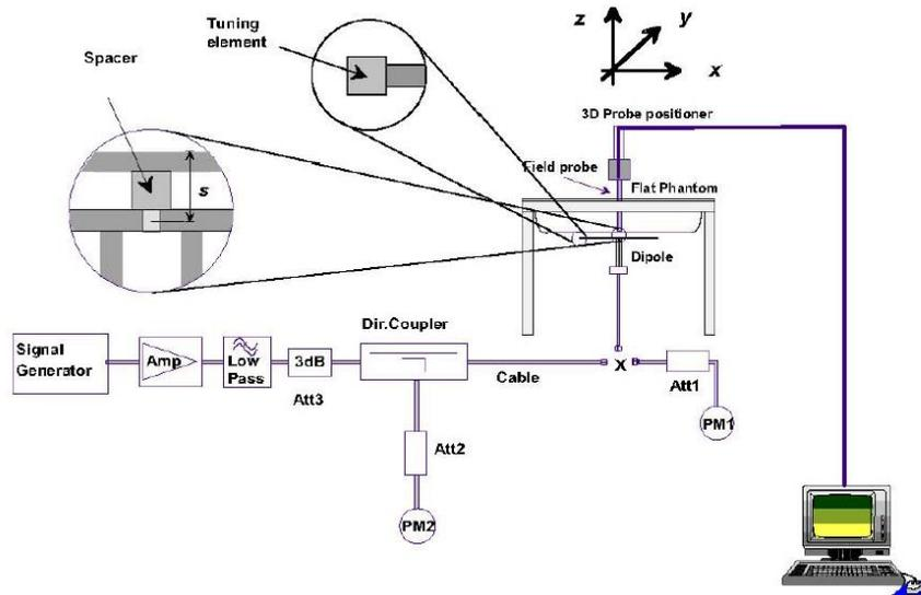
The output power on dipole port must be calibrated to 24 dBm (250mW) before dipole is connected.
