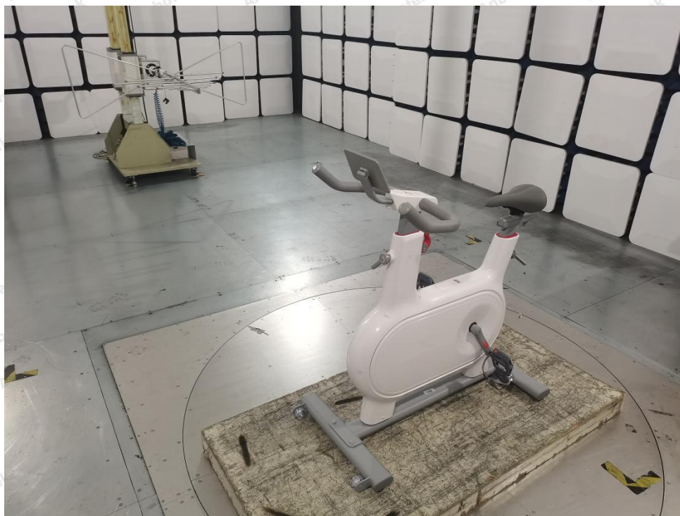
Photo of Radiation Emission Test
