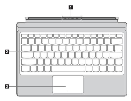
**Pogo pin with guide pin**Connect the tablet to the keyboard Folio and secure it in the installation position.
