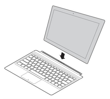
**Note:** Tablet-keyboard folio tongue has strong magnetic force, so as to easily connect with and secure the tablet.
