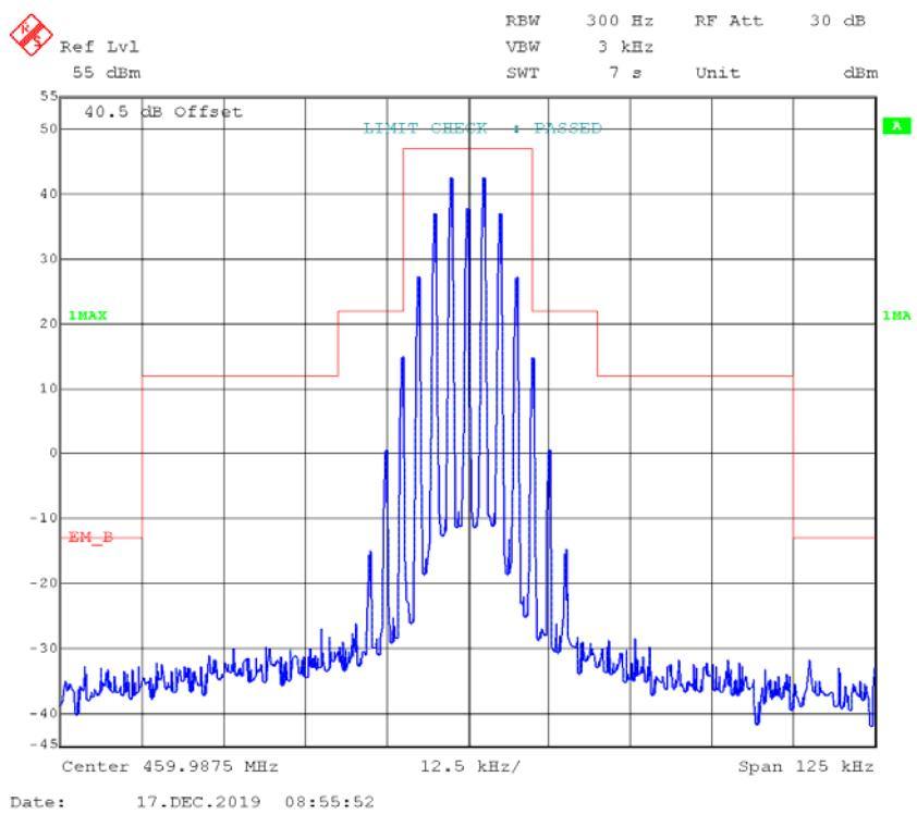
**FM,25kHz,Low Power - Frequency 459.9875 MHz:****99% Occupied & 26 dB Bandwidth**
