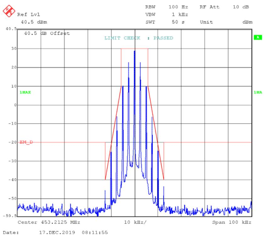
**4FSK,12.5kHz,High Power - Frequency 453.2125 MHz:****99% Occupied & 26 dB Bandwidth**
