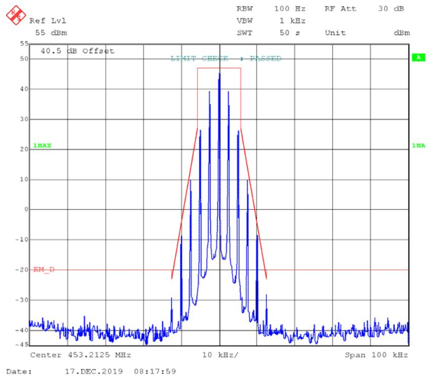
**FM,12.5kHz,Low Power - Frequency 453.2125 MHz:****99% Occupied & 26 dB Bandwidth**
