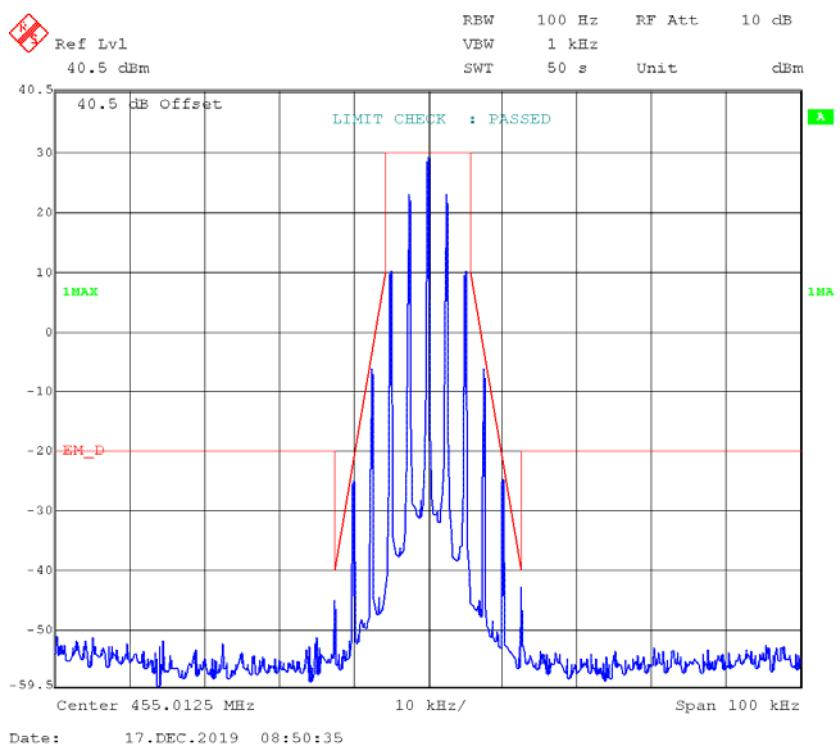
**FM,25kHz,High Power - Frequency 455.0125 MHz****: 99% Occupied & 26 dB Bandwidth**
