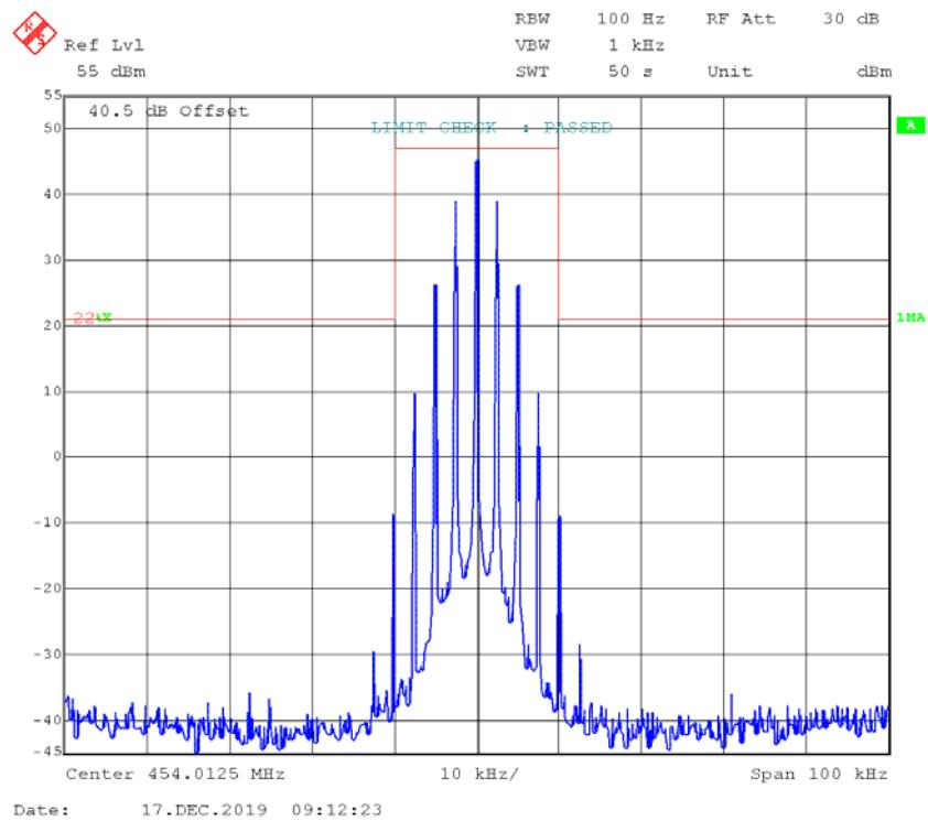
**FM,12.5kHz,Low Power - Frequency 454.0125 MHz:****99% Occupied & 26 dB Bandwidth**
