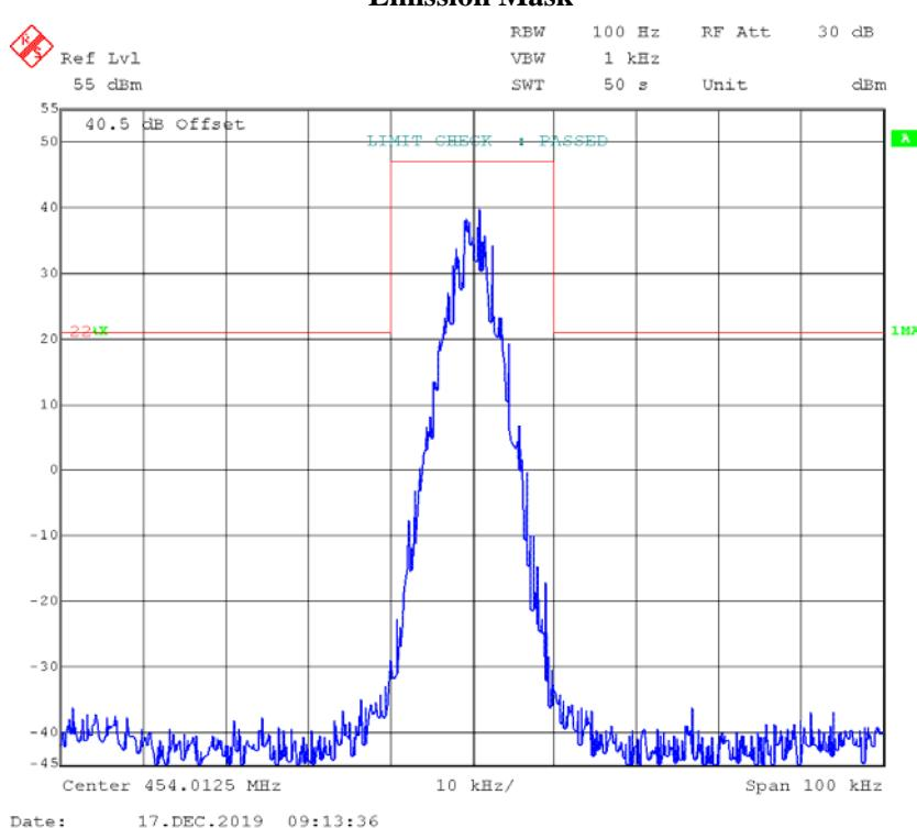
**4FSK,12.5kHz,Low Power - Frequency 454.0125 MHz:****99% Occupied & 26 dB Bandwidth**
