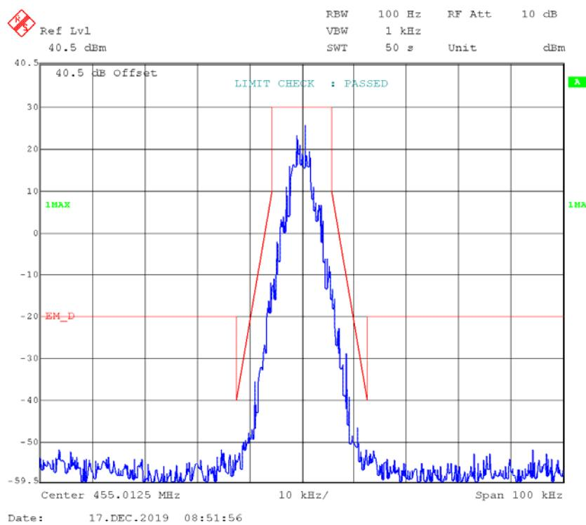
**part 22:****FM,12.5kHz,High Power - Frequency 454.0125 MHz:****99% Occupied & 26 dB Bandwidth**
