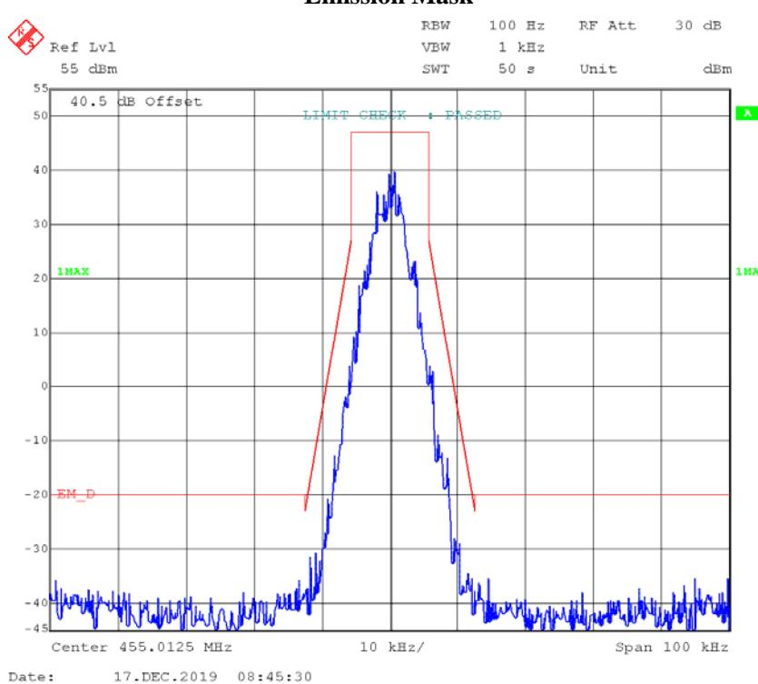
**4FSK ,12.5kHz, Low Power - Frequency455.0125 MHz:****99% Occupied & 26 dB Bandwidth**
