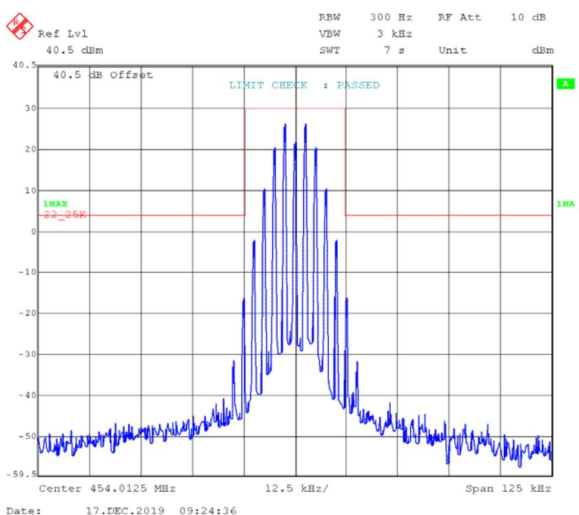
**4FSK,12.5kHz,High Power - Frequency 454.0125 MHz:****99% Occupied & 26 dB Bandwidth**
