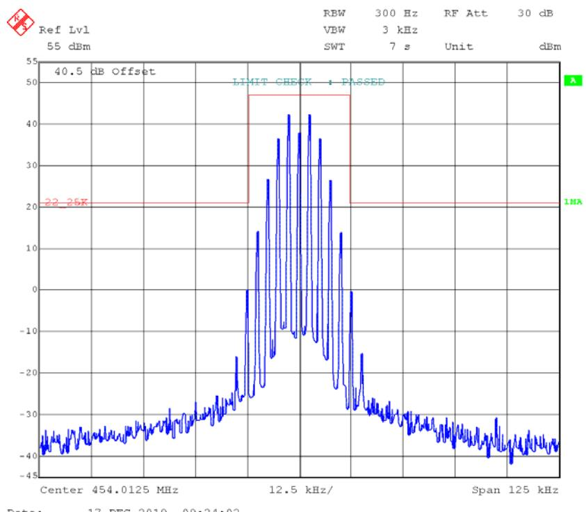
**FM,25kHz,Low Power - Frequency 454.0125 MHz:****99% Occupied & 26 dB Bandwidth**
