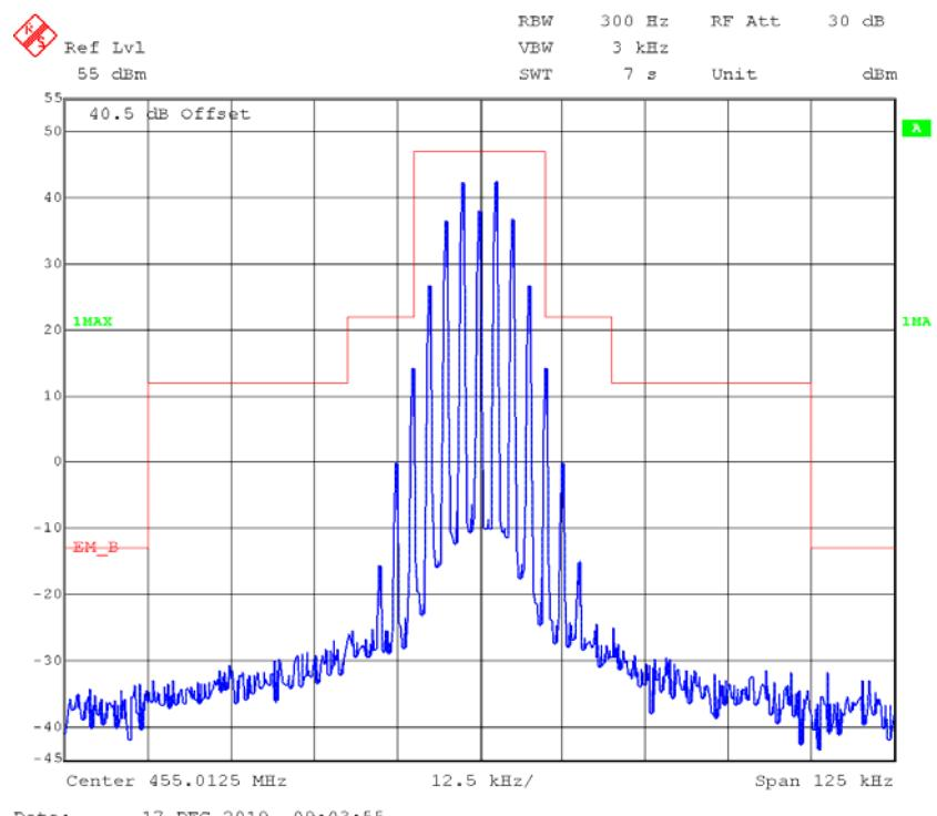
**FM,25kHz,Low Power - Frequency 455.0125 MHz:****99% Occupied & 26 dB Bandwidth**
