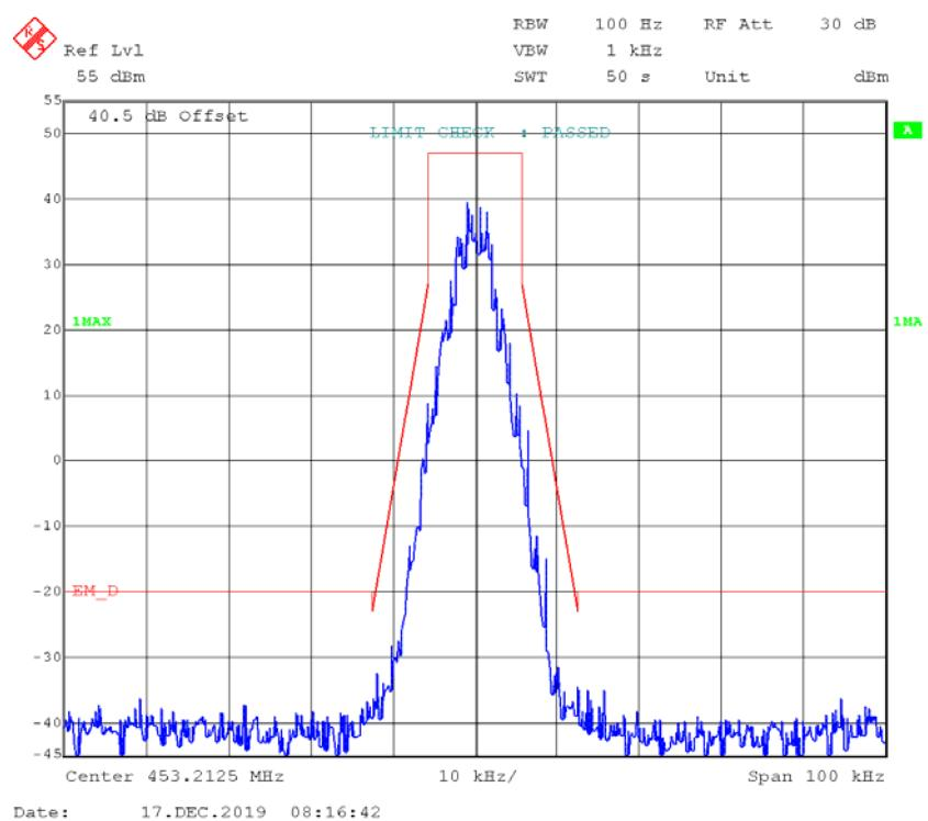
**4FSK,12.5kHz,Low Power - Frequency 453.2125 MHz:****99% Occupied & 26 dB Bandwidth**
