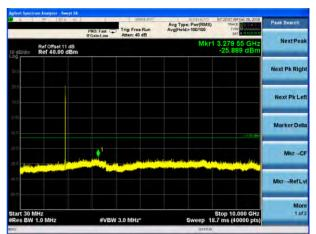
Conducted Emission Transmitting Mode CH 9400 10GHz – 20GHz
