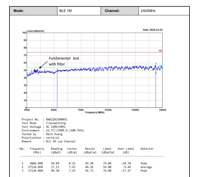
Remarks: Factor = Antenna factor + Cable loss - Preamp gain
