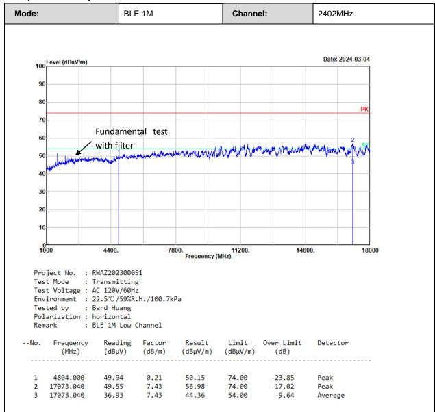
Remarks: Factor = Antenna factor + Cable loss - Preamp gain
