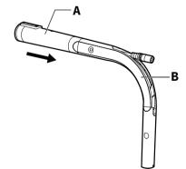
2. Insert the Second Extension (B) onto the Wall Mount Cover (D), ensuring that the slot is correctly aligned.
