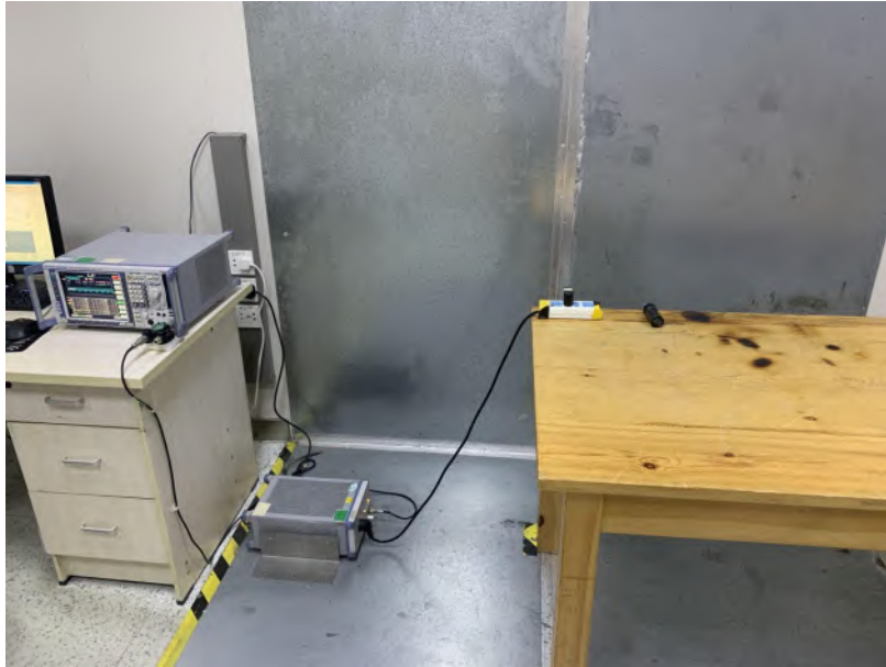
Radiated Emissions From 30M-1GHz
