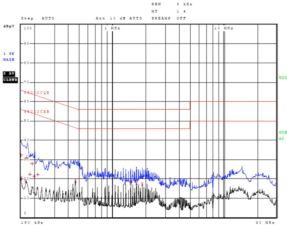
Figure Two AC Line Conducted Emissions Line 2
