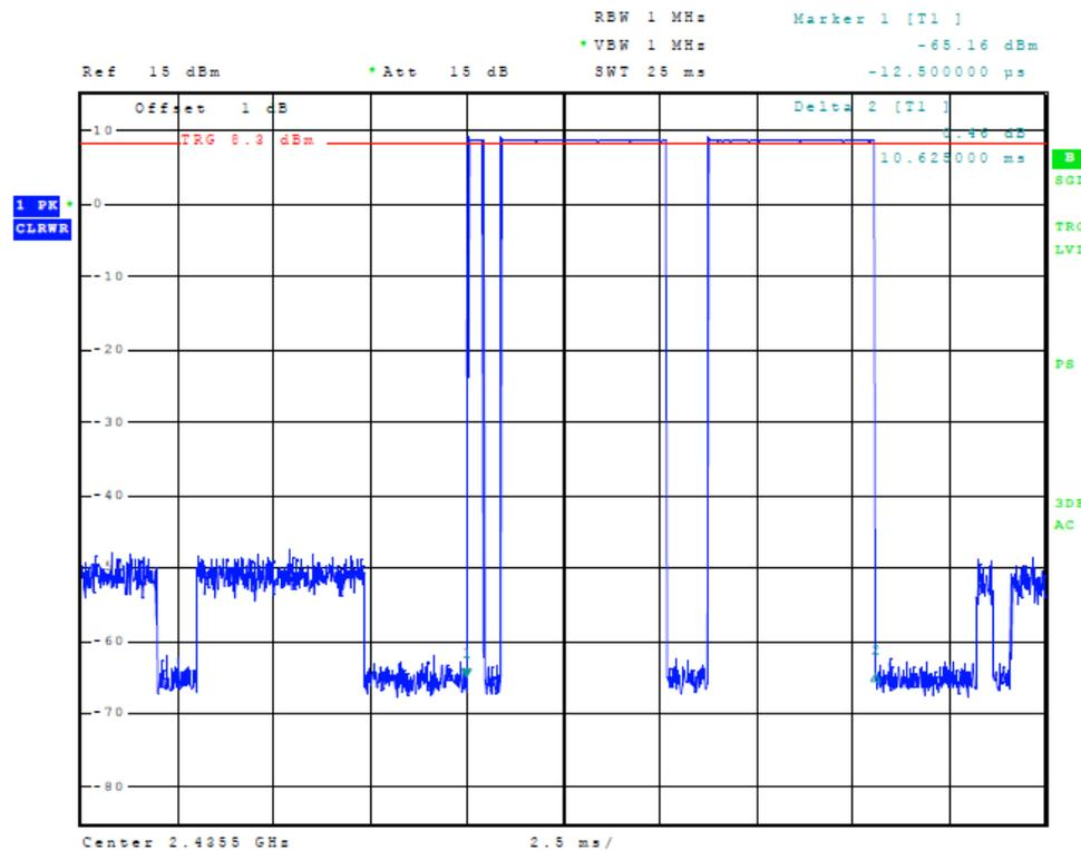
**Figure Five of Antenna Port Conducted Emissions (Dwell Time on Channel)**
