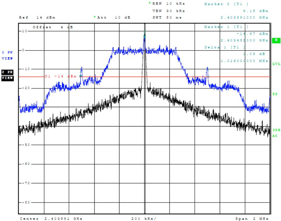
Figure Seven of Antenna Port Conducted Emissions (Occupied Bandwidth 2403)
