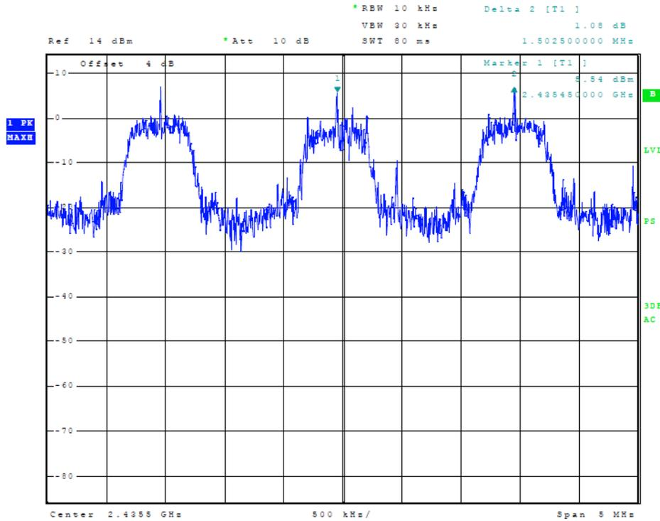
**Figure Four of Antenna Port Conducted Emissions (Channel Separation)**
