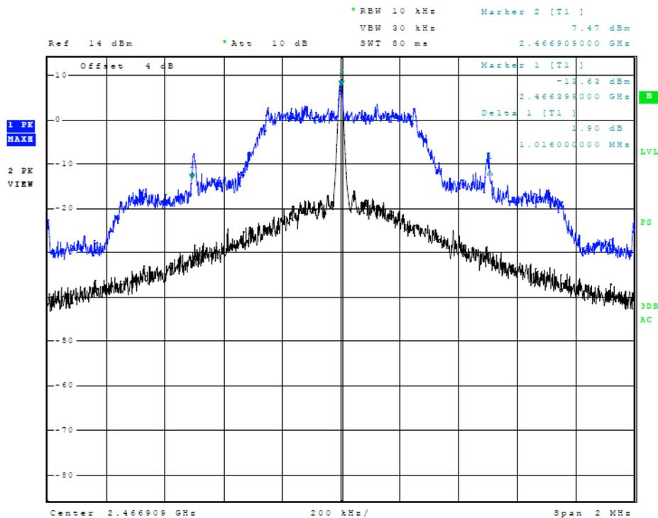
**Figure Nine of Antenna Port Conducted Emissions (Occupied Bandwidth 2466)**
