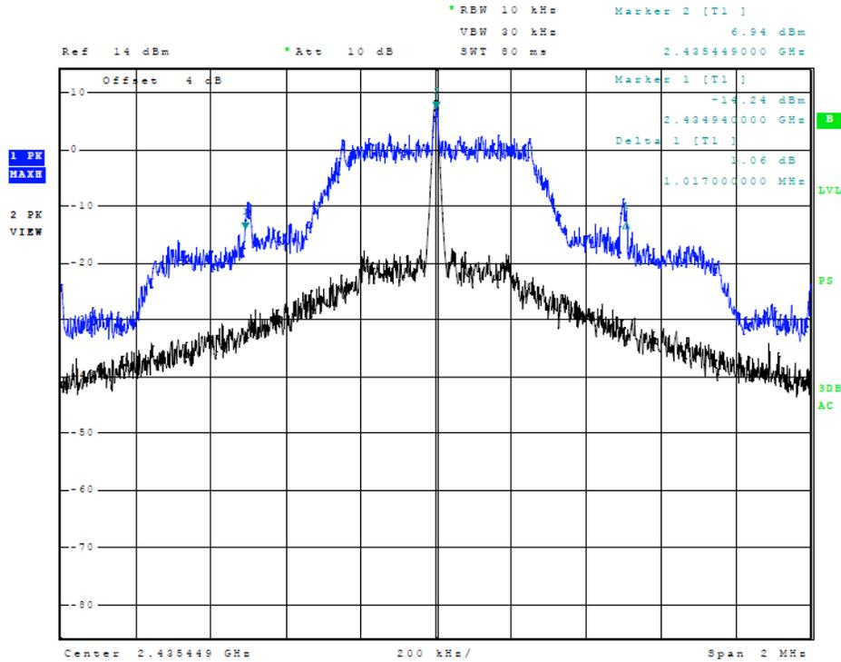
**Figure Eight of Antenna Port Conducted Emissions (Occupied Bandwidth 2435)**
