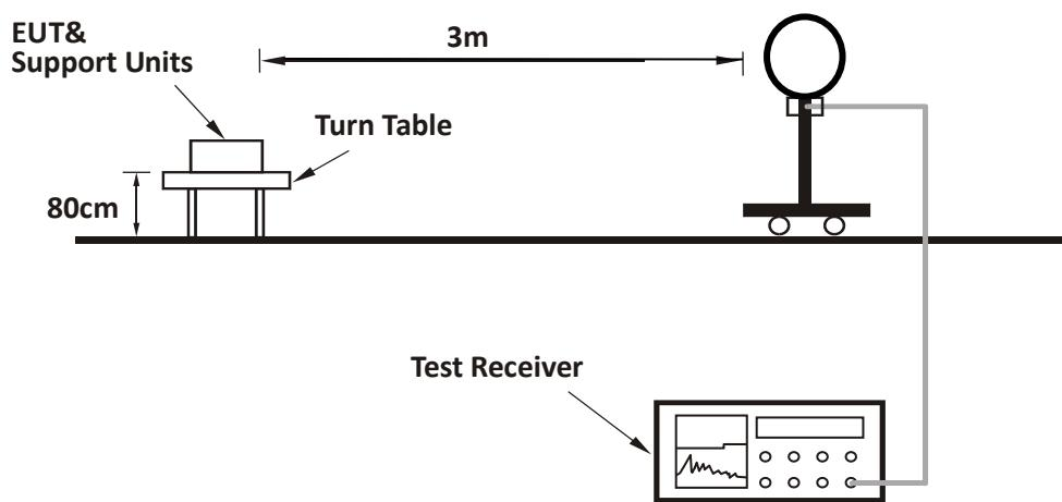
**For Radiated emission 30MHz to 1GHz:**
