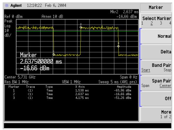
This shows a transmit duty cycle of (4.175-2.637)/(4.175-1.538) or 0.583. This corresponds to a difference of 2.34dB between the power during the burst and the mean power level..
