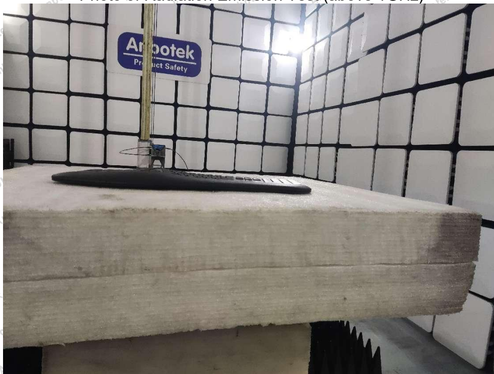
Photo of Radiation Emission Test (above 1GHz)
