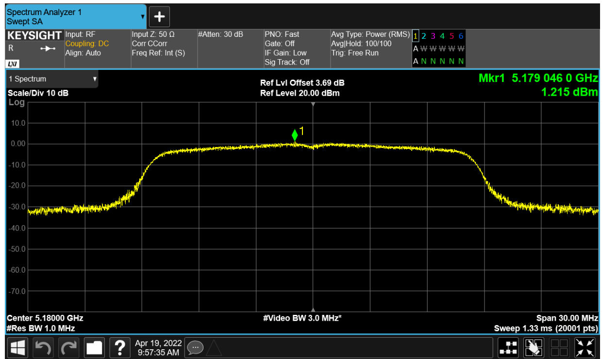
PSD NVNT a 5200MHz Ant1
