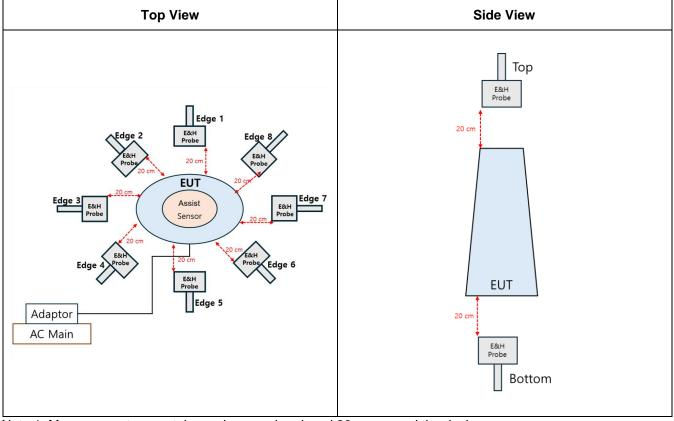
Note 1. Measurements were taken using a probe placed 20 cm around the device. Note 2. Edge 1 is where the EUT's 'SAMSUNG' phrase is written.
