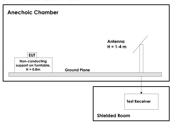
This test setup is used for all radiated emissions tests. Measuring distance is 3m for all frequencies.
