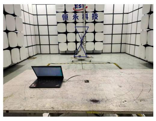
Radiated Test (Above 1GHz)
