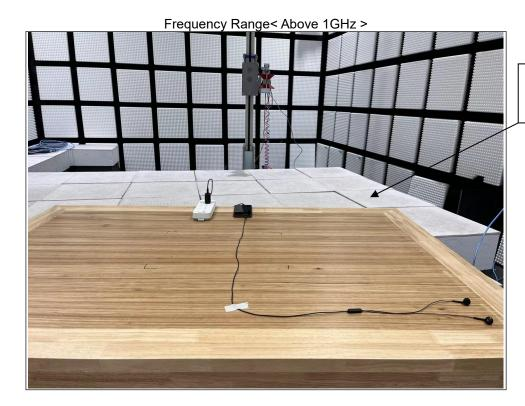
the absorbing material is under the foam
