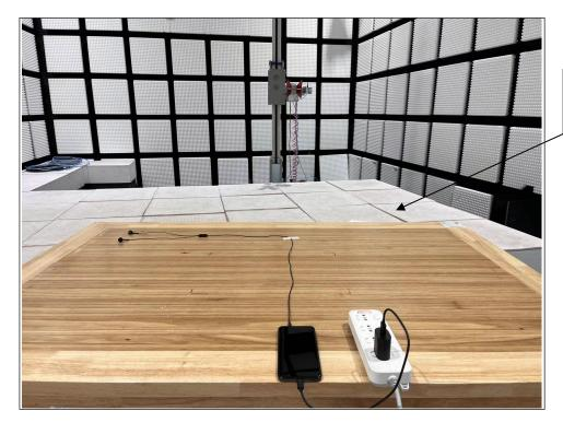
the absorbing material is under the foam
