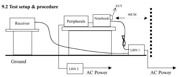
The EUT are connected to the main power through a line impedance stabilization network (LISN). This provides a 50 ohm/50uH coupling impedance for the measuring equipment. The peripheral devices are also connected to the main power through a LISN that provides a 50ohm/50uH coupling impedance with 50ohm termination.
