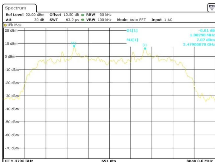
**EDR (8DPSK): Low Channel**
