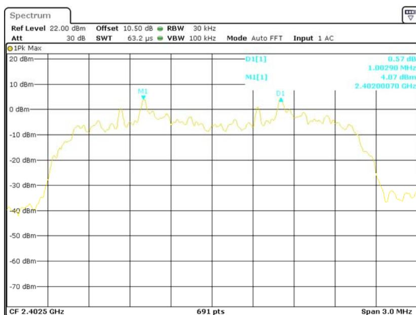
**EDR ( $\pi/4$ -DQPSK): Middle Channel**
