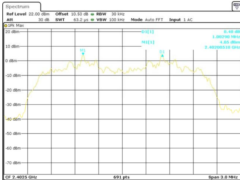
**EDR (8DPSK): Middle Channel**
