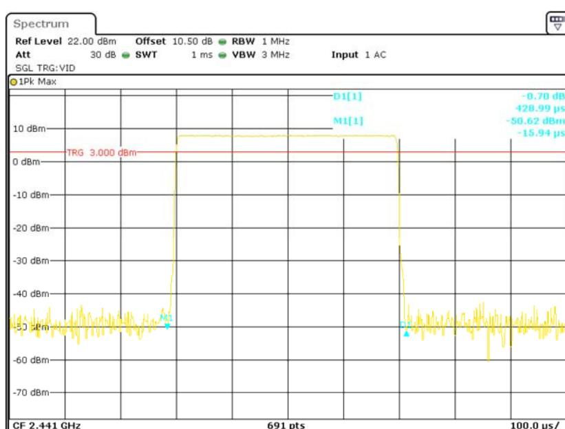
**Pulse time, High Channel, DH1**
