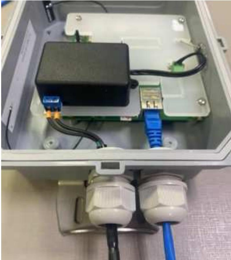
Figure: Ethernet Connection and power cables
