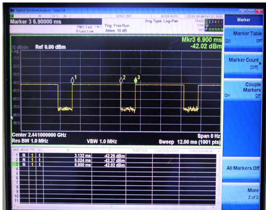
Time-domain plot for Bluetooth transmission signal
