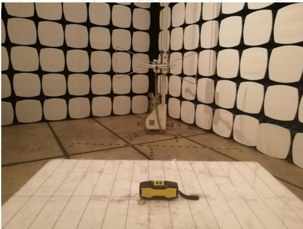
FCC RADIATED EMISSION TEST SETUP
