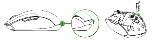
2. Close the top cover and insert the wireless USB dongle into the USB port of your PC.
