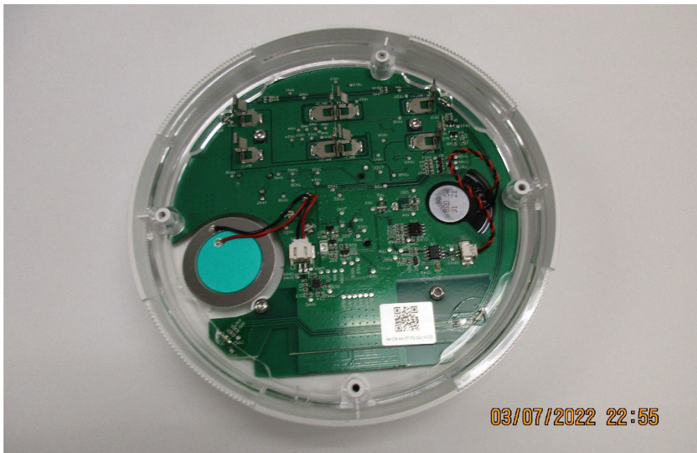
Figure 2 PCB without battery holder
