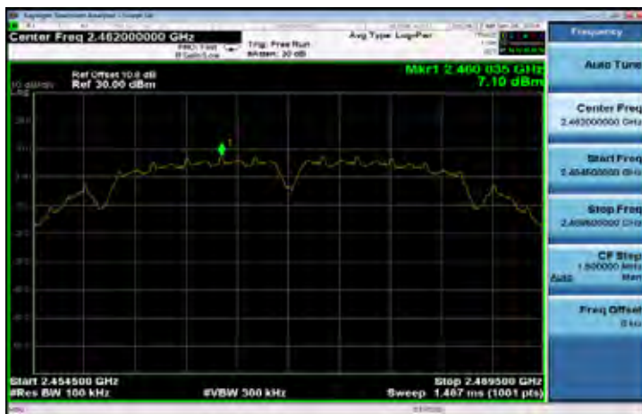
802.11b Reference Level of Emission Limit (CH-High)
