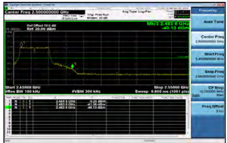
802.11g: Band Edges Test Data CH-High
