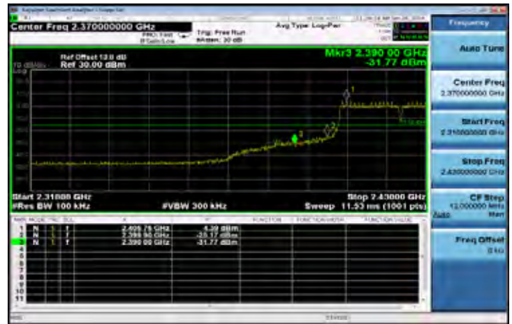
802.11n_HT40: Band Edges Test Data CH-High
