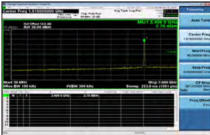
802.11n_HT20: Spurious Emission Test Data CH-Low
