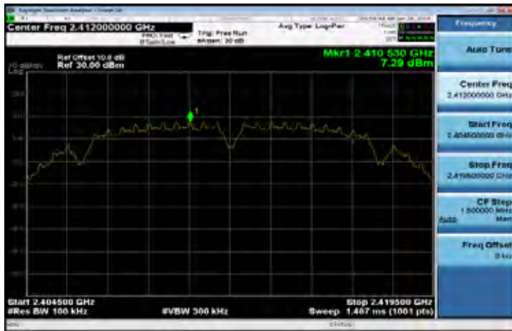
802.11b Reference Level of Emission Limit (CH-High)
