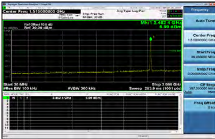
802.11b: Spurious Emission Test Data CH-High
