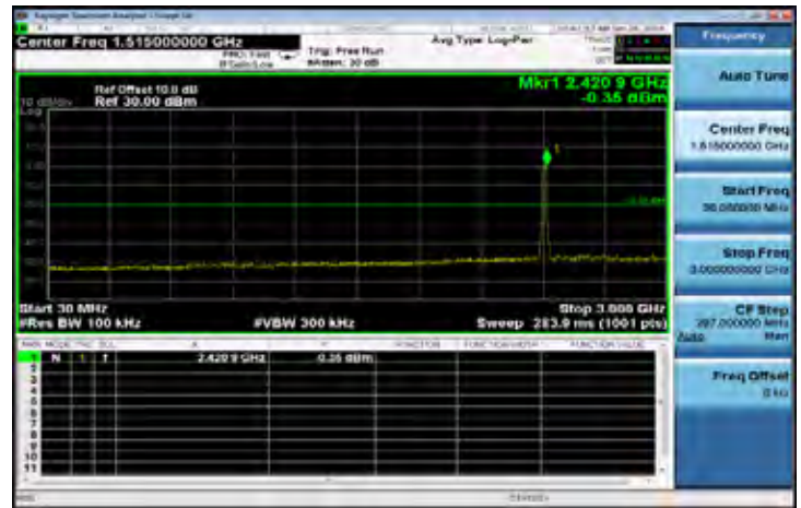
802.11g: Spurious Emission Test Data CH-Low
