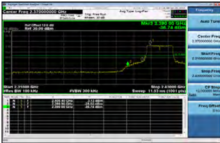
802.11n_HT20: Band Edges Test Data CH-High
