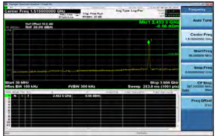
802.11g: Spurious Emission Test Data CH-High
