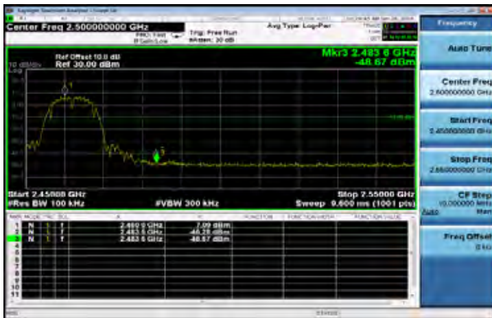
802.11b: Band Edges Test Data CH-High
