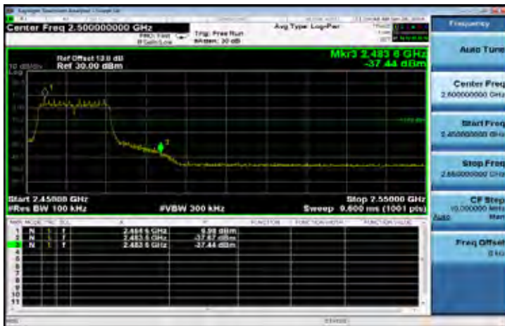
802.11n_HT20: Band Edges Test Data CH-High
