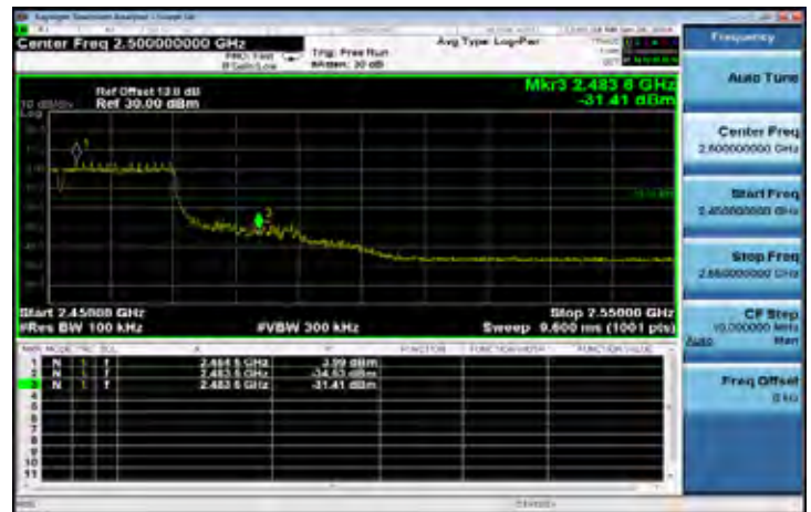
802.11n_HT40: Band Edges Test Data CH-High
