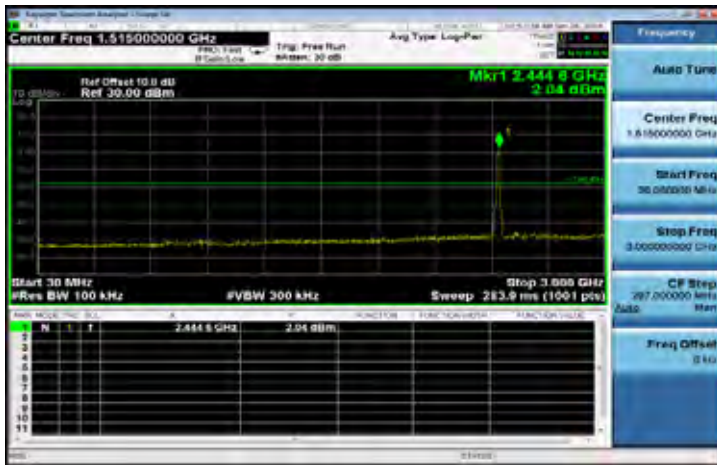
802.11g: Spurious Emission Test Data CH-Mid
