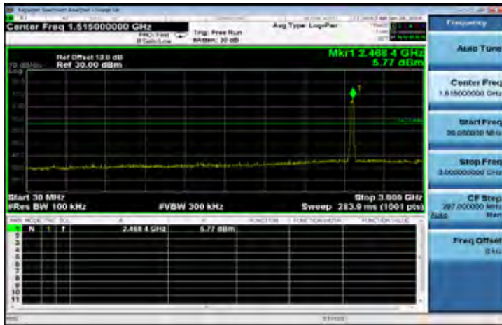
802.11n_HT20: Spurious Emission Test Data CH-High
