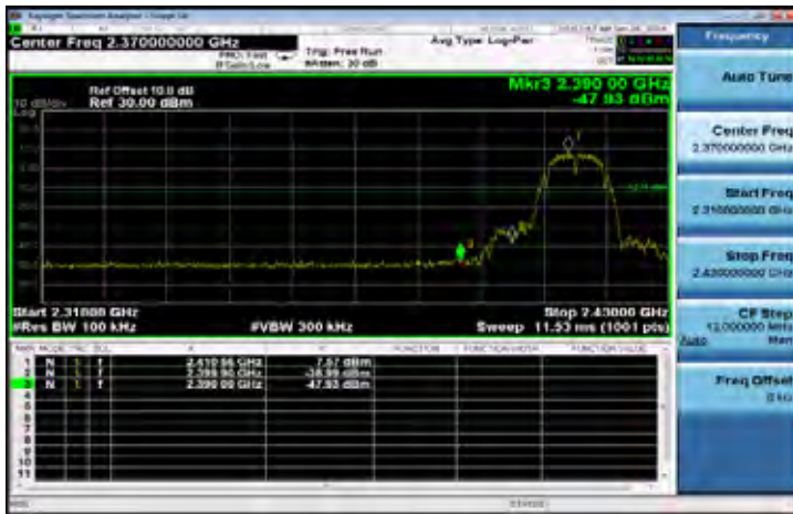
802.11b: Band Edges Test Data CH-High
