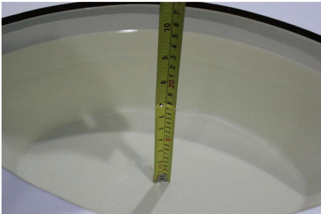
Picture 7-2: Liquid depth in the Flat Phantom(5GHz)
