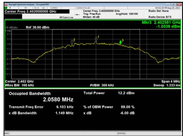
Bluetooth LE (2M) Carrier frequency (MHz): 2440
