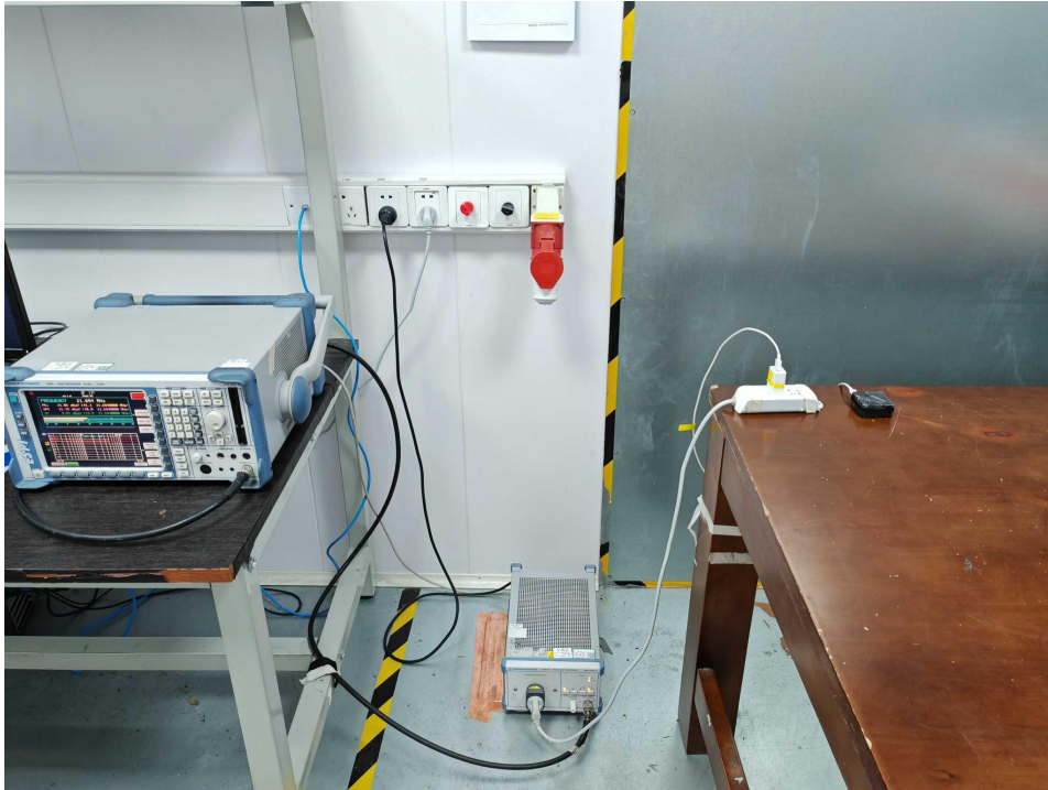
Conducted emissions at AC power line (150kHz-30MHz)
