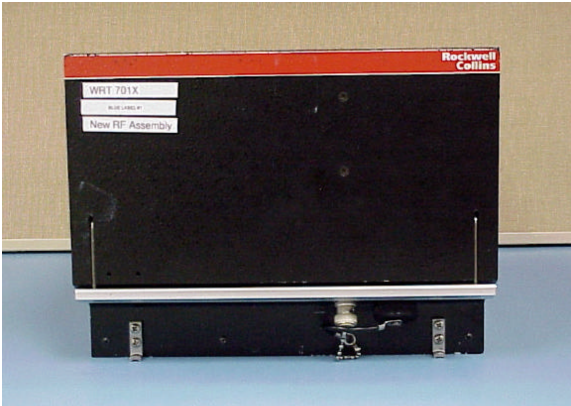
Figure C-3. WRT-701 Front Panel
