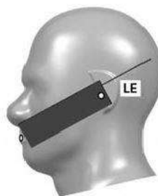
Fig 9.2.2 Handset vertical and horizontal reference lines—“clam-shell case”
