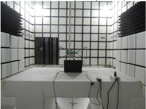
Radiated Emission Set up Photos (Above 1GHz)
