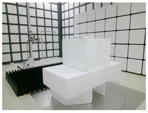
Description: Radiated Emission Test Setup for above 1GHz (Wi-Fi 5G)
