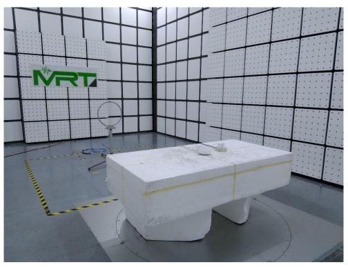
Description: Radiated Emission Test Setup for 9kHz~30MHz
