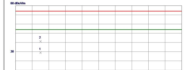
(MHz) Reading Correct Measure No. Freq. Limit Margin Level Factor ment dBuV/m dB dBuV/m dBuV/m dB Detector Comment 1 \* 4818. 5000 24. 65 4.23 28.88 54.00 -25.12AVG 2 4821.8000 37.04 4.25 41.29 74.00 -32.71Peak
