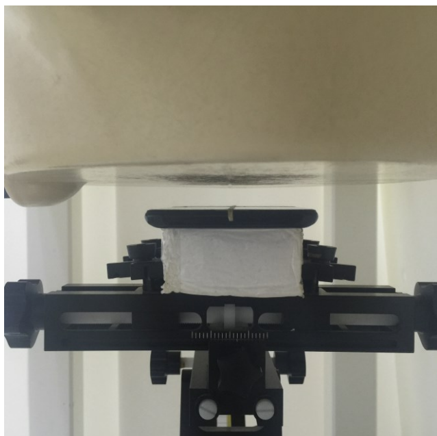
Front, Test Separation 15 mm
