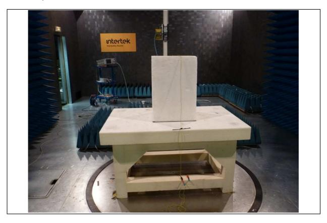
Test Setup Photo - Radiated emissions 7 GHz to 18 GHz
