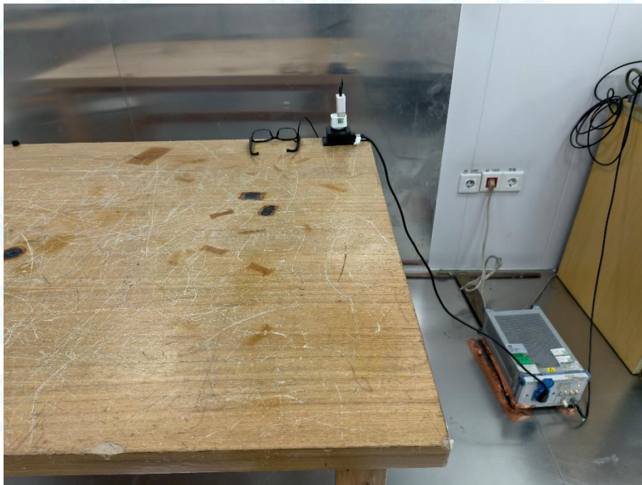
Photo of Setup for Conducted Emission
