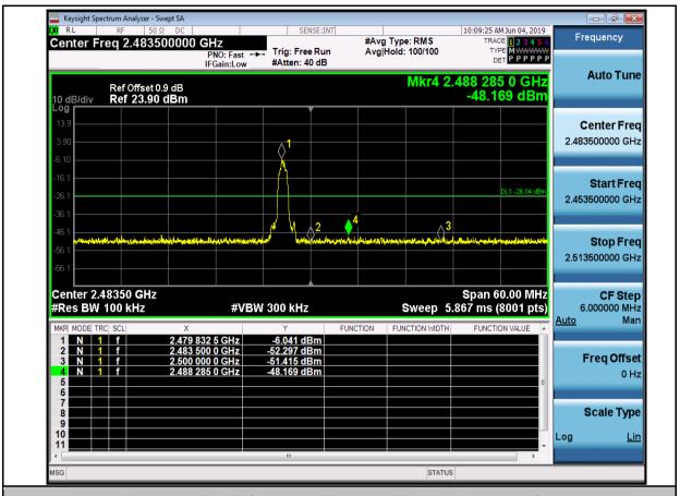
Band-edge for RF Conducted Emissions\_DH5\_2402\_Hopping On
