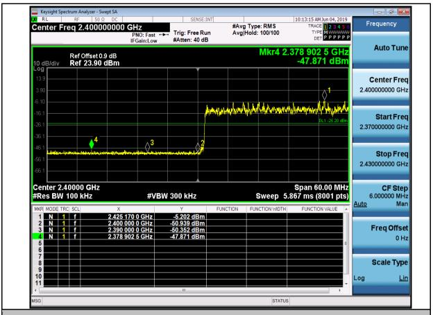
Band-edge for RF Conducted Emissions 2DH5 2480 Hopping On
