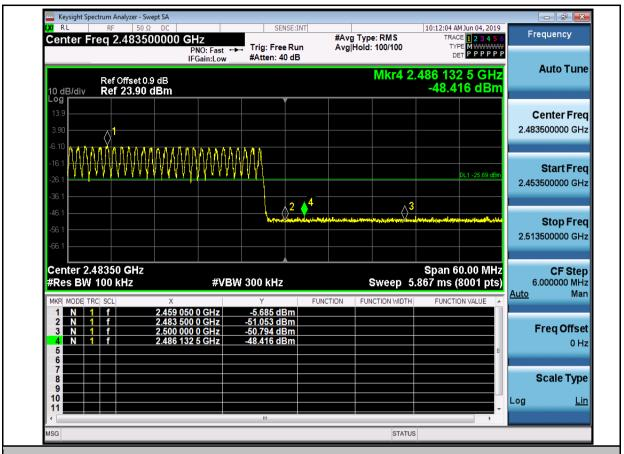
Band-edge for RF Conducted Emissions 2DH5 2402 Hopping On
