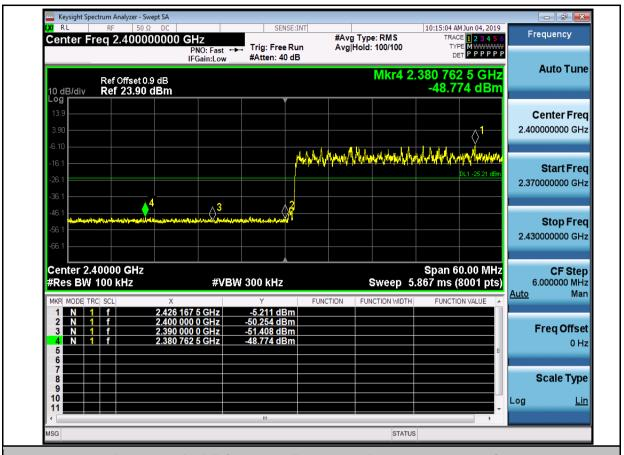
Band-edge for RF Conducted Emissions\_3DH5\_2480\_Hopping On
