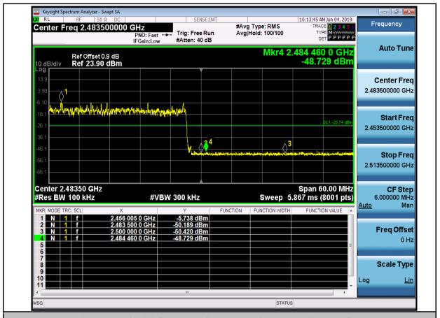
Band-edge for RF Conducted Emissions\_3DH5\_2402\_Hopping On
