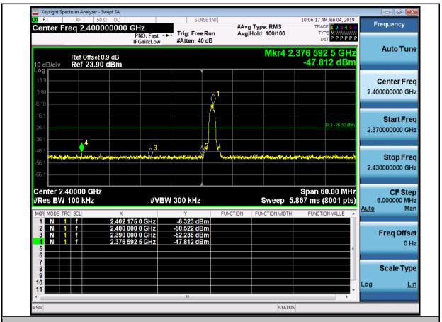
Band-edge for RF Conducted Emissions 3DH5 2480 Hopping Off
