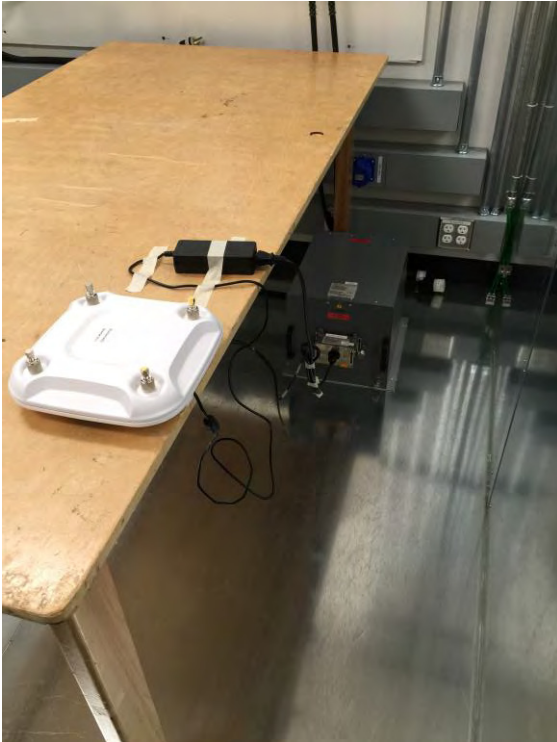
AIR-CAP3702P-B-K9 AC Conducted Emissions setup photo
