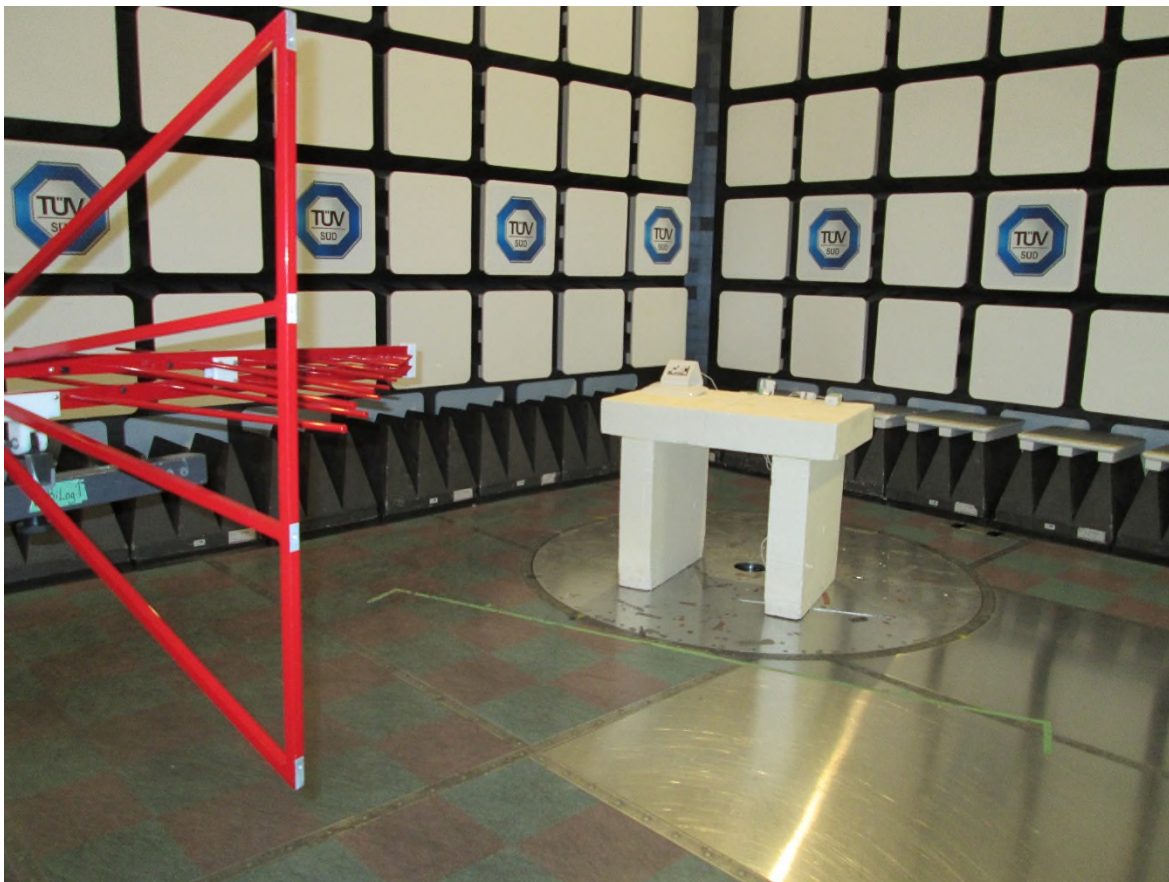
Test setup photo 2 Radiated measurements, 30 MHz – 1 GHz
