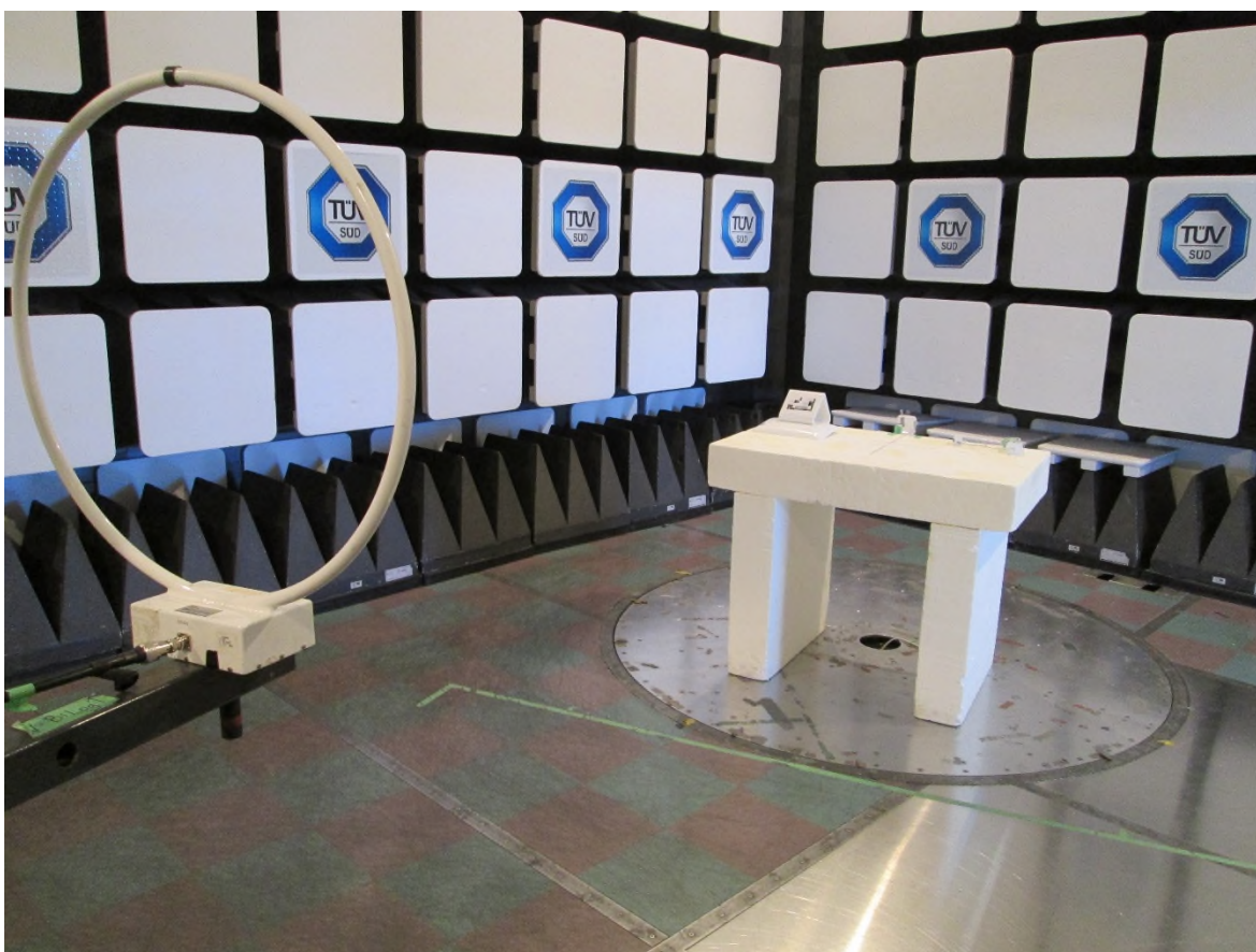
Test setup photo 1 Radiated measurements, 9 kHz – 30 MHz
