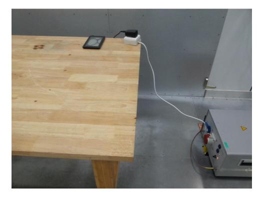
Radiated Emission Test Below 1GHz
