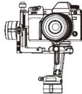
Mount the camera horizontally
