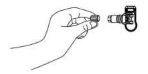
Step 1. Remove the valve caps and nuts from the valve stems one by one.
