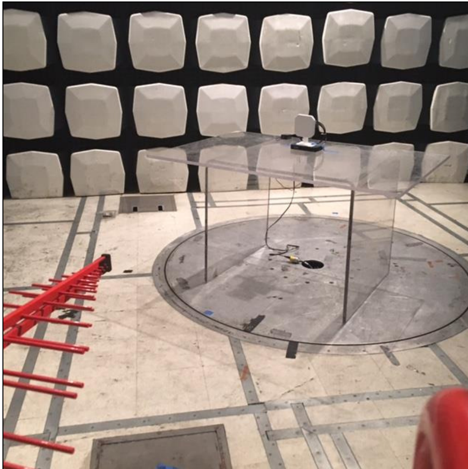
Photograph 2. Radiated Spurious Emissions, Test Setup
