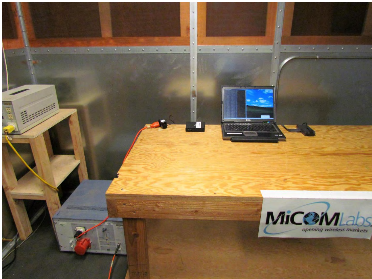
Conducted Emissions ACDC powered configuration
