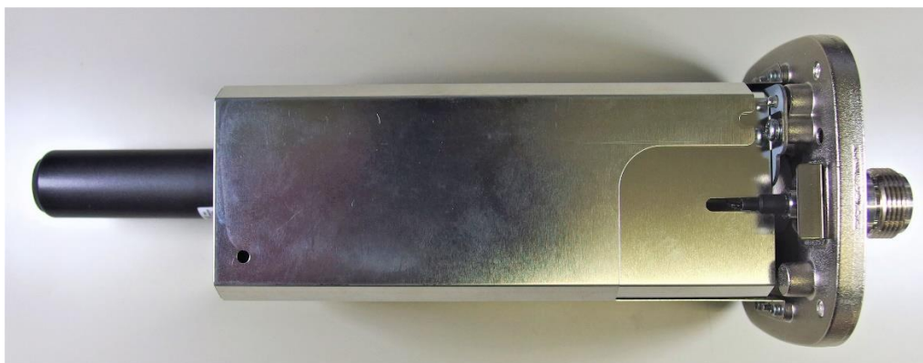
AH-41 RX Unit with chassis, antenna and shield Side A
