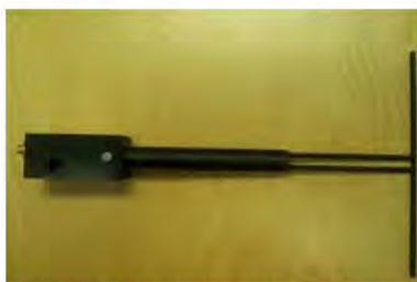
Figure 1 – MVG COMOSAR Validation Dipole
