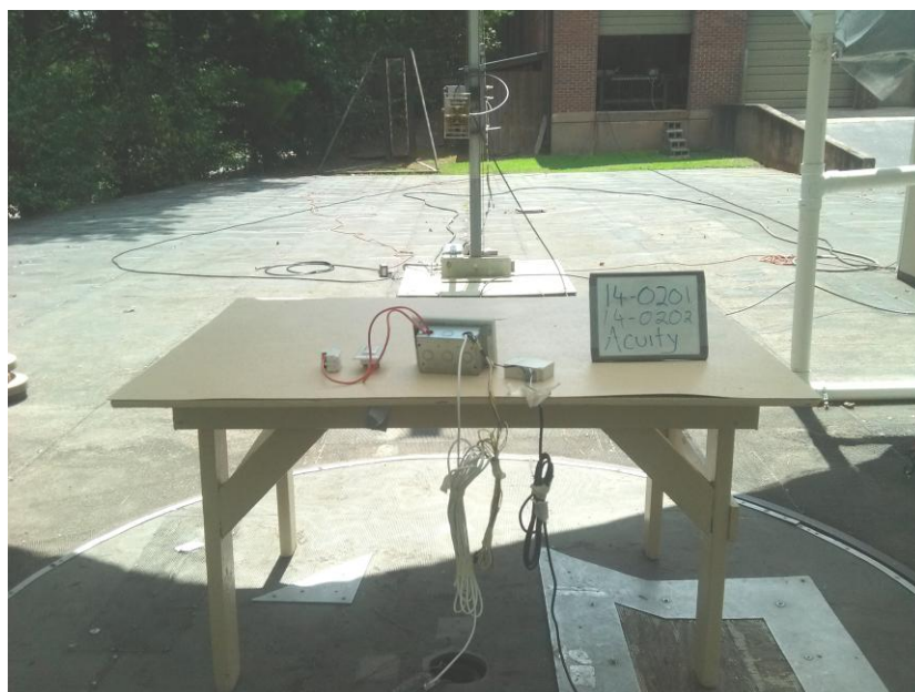
Photo 4- Radiated Emissions Test Setup, 1GHz and Above, Back
