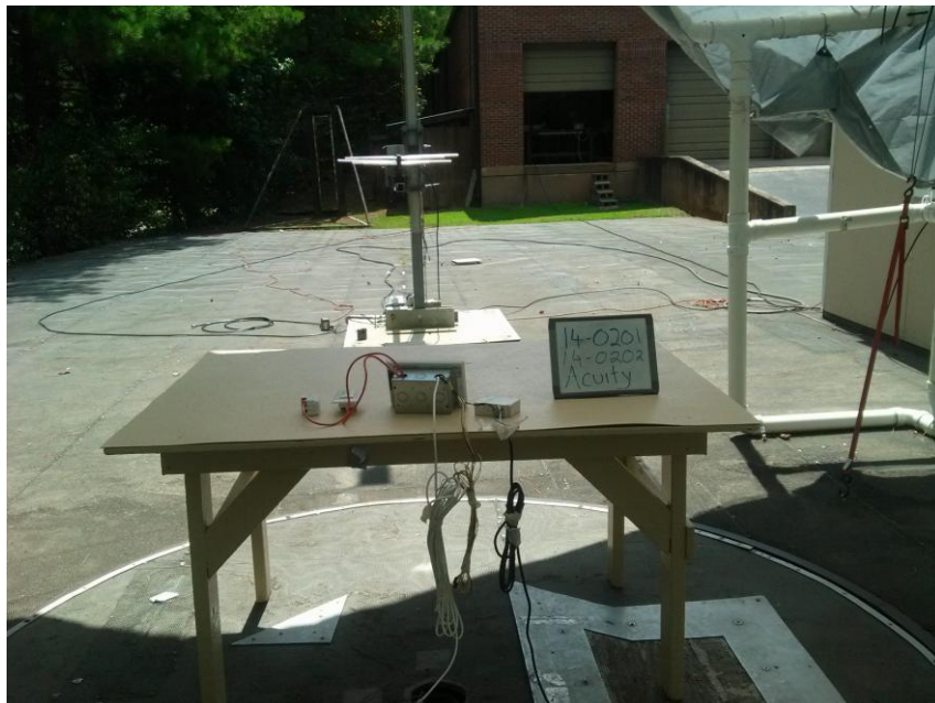
Photo 3- Radiated Emissions Test Setup, 200 MHz to 1000 MHz, Back
