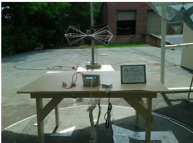
Photo 2- Radiated Emissions Test Setup, 30 MHz to 200 MHz, Back
