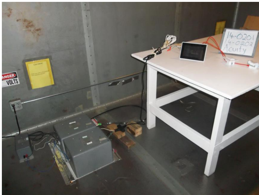
Photo 6- Conducted Emissions Test Setup
